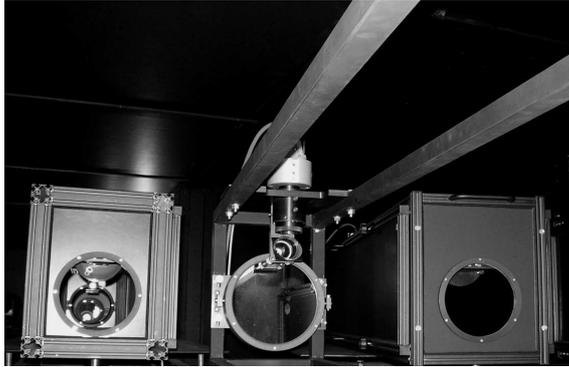
Figure 5: The main camera objectives  $\phi$  200 mm, f 2500 mm can be seen in the center through the metallic (usually covered by shielding) construction. Above it is the Vosskuhler CCD camera.
