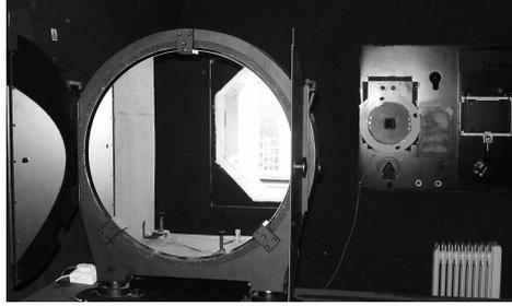
Figure 3: The HSFA main objective  $\phi$  50 cm, f 35 m is in the left. To the right is the entrance slit of the spectrograph with the rectangular reflecting mirror for the slit-jaw.
