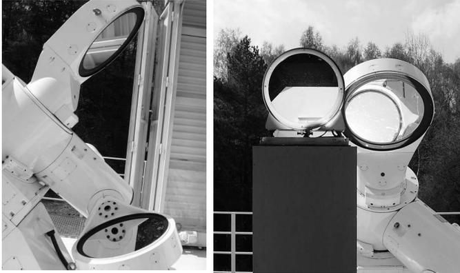
Figure 2: Left: The Jensch-type coelostat consisting of two 60 cm flat mirrors is located 4 – 6 m above the ground and is covered by a moving metallic shelter. Right: A look to the  $\phi$  32 cm flat mirror of the telescope and the upper mirror of the coelostat.
