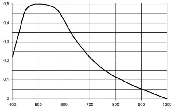
Figure 6: Quantum efficiency of the used CCD camera chip as a function of wavelength.
