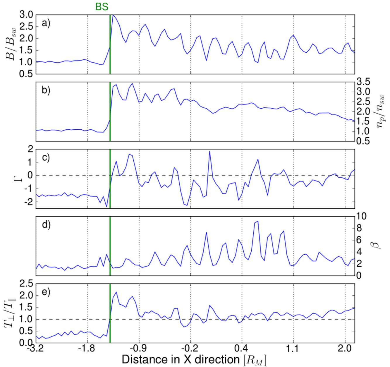
**Figure 6.** Data from the SIMF simulation along a flowline crossing the dawn region suspected of mirror waves. The flowline is indicated in the Figure 5 by the black dashed line. Panel a) gives a magnetic field amplitude normalized to the solar wind magnetic field, panel b) proton density normalized to the solar wind density, panel c)  $\Gamma$ , panel d)  $\beta$ , and panel d) temperature anisotropy. The green solid vertical line denotes the position of a bow shock.
